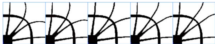
Fig. 8: Geometries produced by the parametric model, with FEM files being produced for structural analysis
